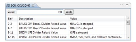
In this view you can set the individual values in the register, either by selecting a value from a drop-down box or by simply entering a value depending on the chosen field. To update the register with the new values, click the **Write** button.
