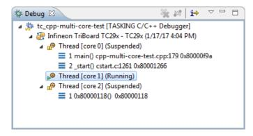
For each of the three TriCore cores of the TC29x a separate thread is started. The example shows the situation where Thread [core 0] is suspended, Thread [core 1] is running and Thread [core 2] is suspended.
