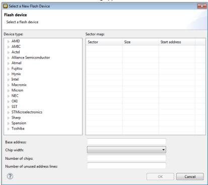
4. In the **Device type** box, expand the name of the manufacturer of the device and select a device.
